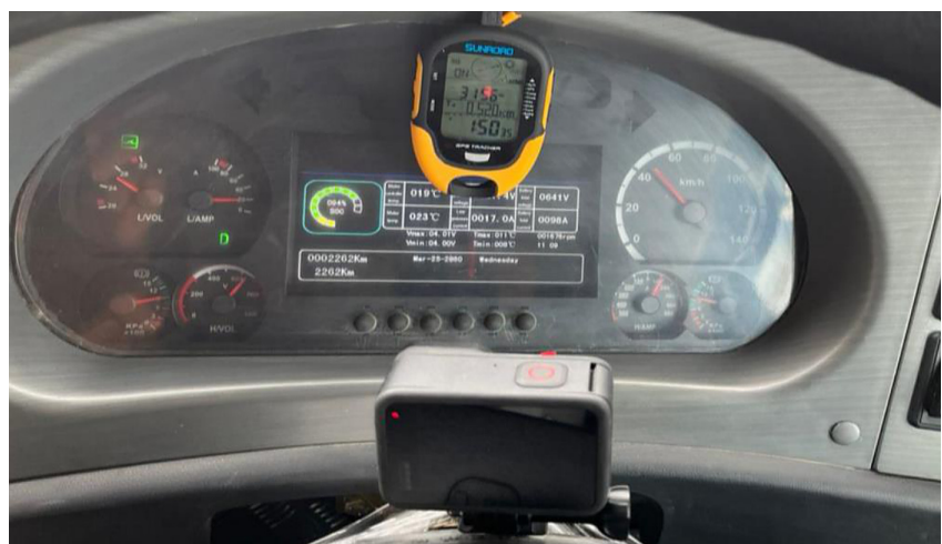
(b) Dashboard with altimeter and video camera
