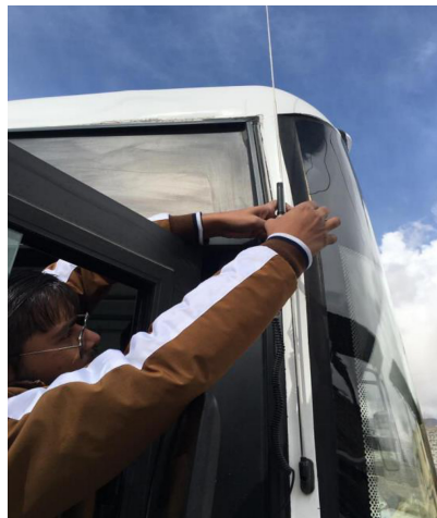
(b) Fixing the external temperature probe
